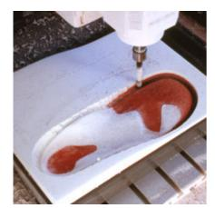
analysis- and construction software for the central insole milling
