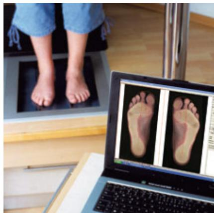
2D-footscan SPEED for the optical ascertainment of significant foot measures and indications
